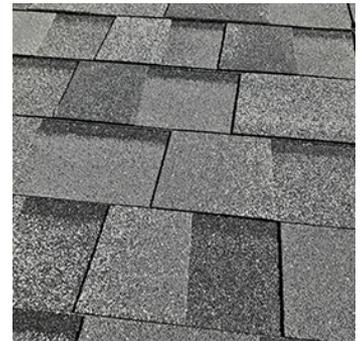
Bitumen shingles have a sturdy glass fibre felt carrier, coated with rubber bitumen (SBS) which makes the product flexible and durable. Granules on the top surface protect the product from the influences of weather. The underside has spots of adhesive.
