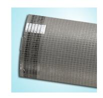
As the product is diffusion-open, a ventilation space is not necessarily required in the roof's structure between the thermal insulation and the underlay, and, consequentially, this space can be used for additional insulation. As there is no ventilation space, heat loss is also reduced, rendering the overall structure more energy-efficient.
